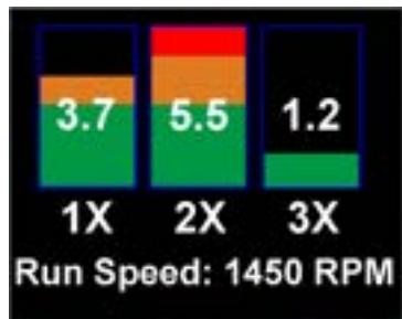
**N.B. in order to perform a vibration analysis it is important that the running speed of the machine is entered correctly. This can be done with the “Setup Wizard” as described in Section 2.3.1 of this user guide, or by using the strobe attachment (see Section 5.1)**
